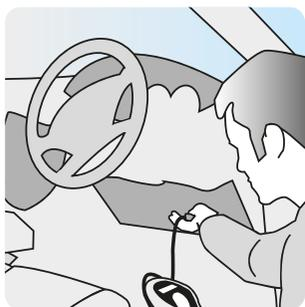
**Step 2:** Connect the data lead on your bluefin to the diagnostic port.
